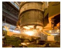
The use of EAFs allows steel to be made from 100% scrap metal feedstock. Therefore. the primary benefit is the substitution of virgin iron which requires much energy to be produced, with scrap that has no emission as it is waste. It is significant that there is a large reduction in specific energy (energy per unit weight) required to produce steel. In addition, modern EAFs are more flexible, being able to vary production to meet
