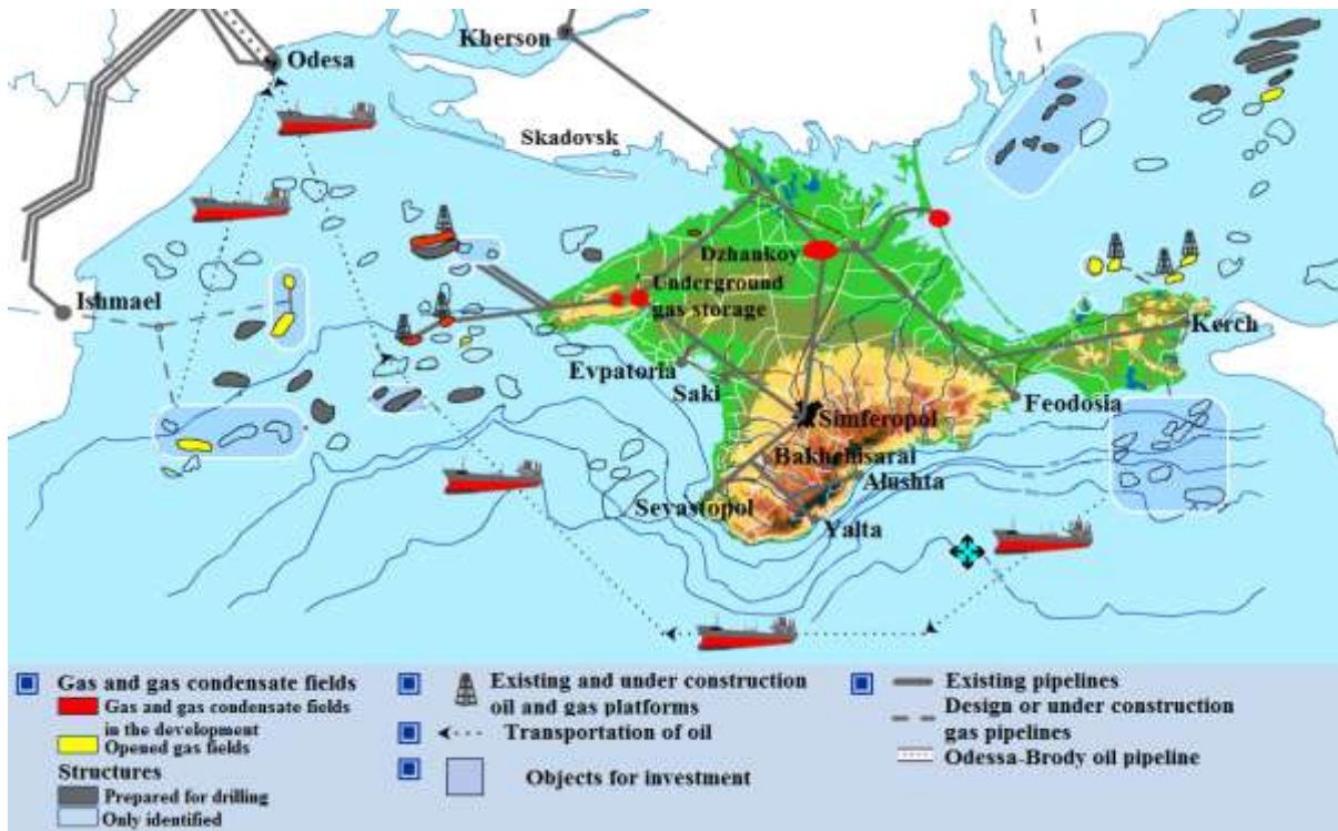
Figure. 2. Scheme of the gas transportation system of NJSC "Chornomornaftogaz"
