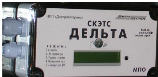
Figure4. On-board system of control over parameters of diesel locomotive operation "Delta SU"
