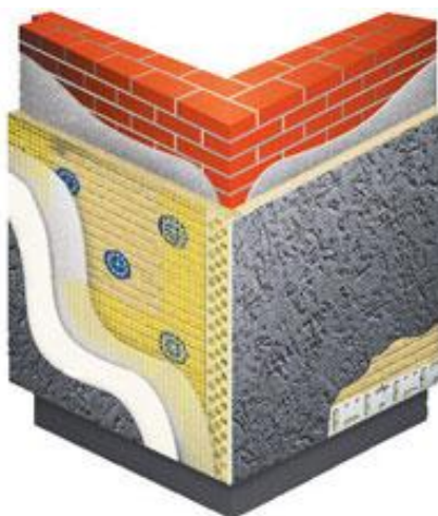
Figure15. Scheme of thermal insulation of external walls
