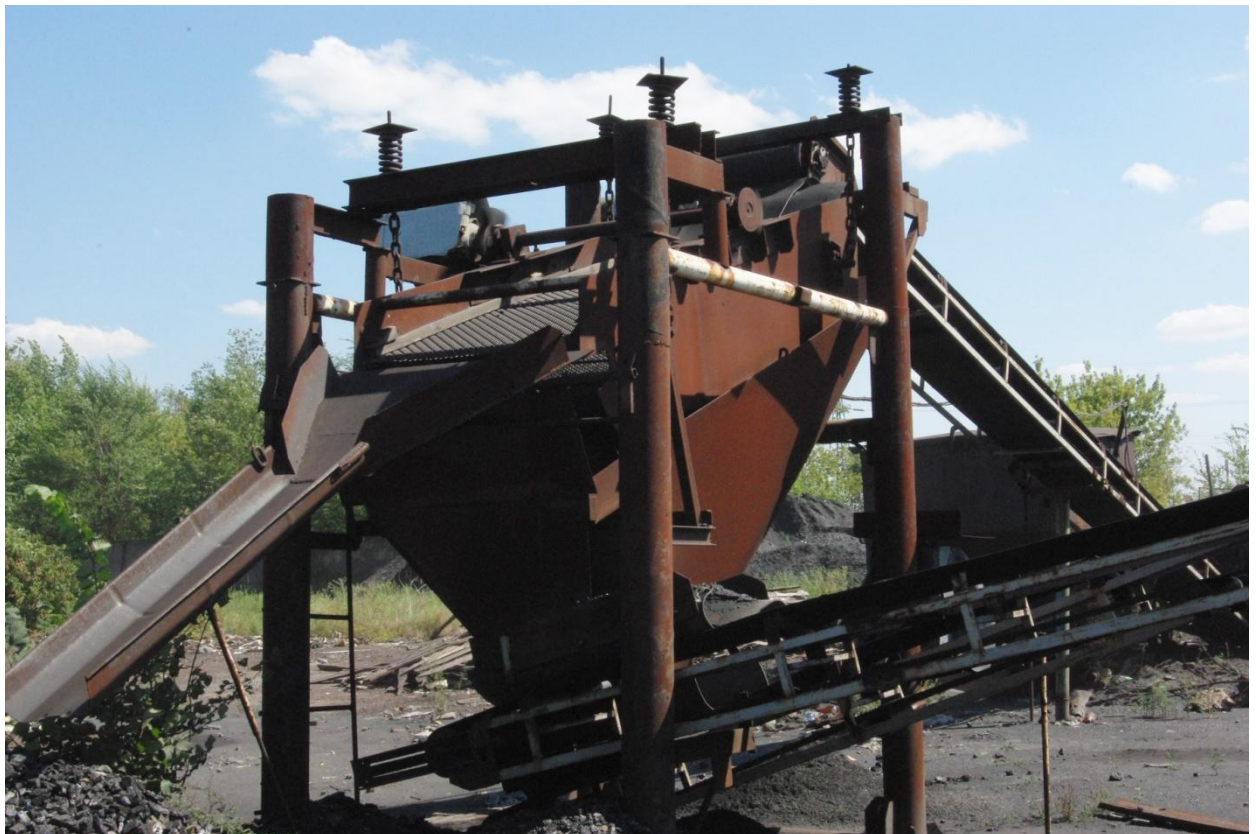
Figure 3 - Machinery for the rock mass sorting
