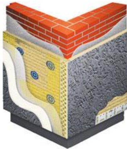
Figure15. Scheme of thermal insulation of external walls
