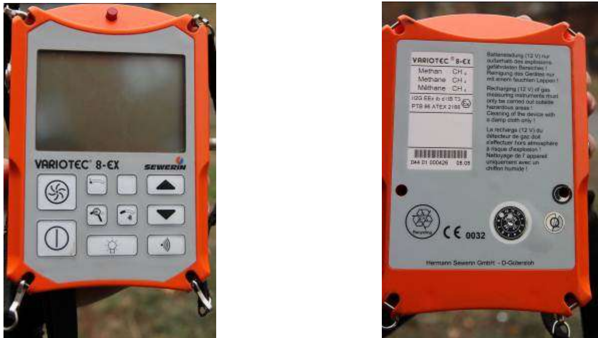
Figure 3. Photo of gas analyzer Variotec® 8-EX.
