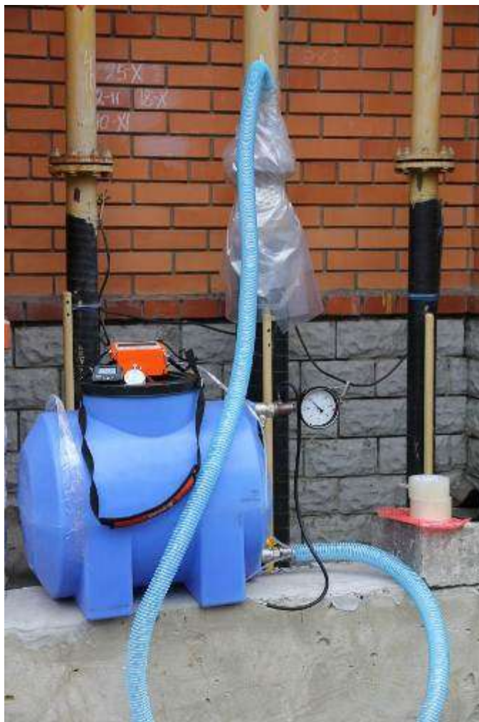
Figure 2. Photo of a device for quantitative measurement of methane leaks
