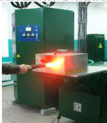
Figure 9. INU-50 industrial-frequency blank heating unit manufactured by “Vnesh-Komplekt” LLC
