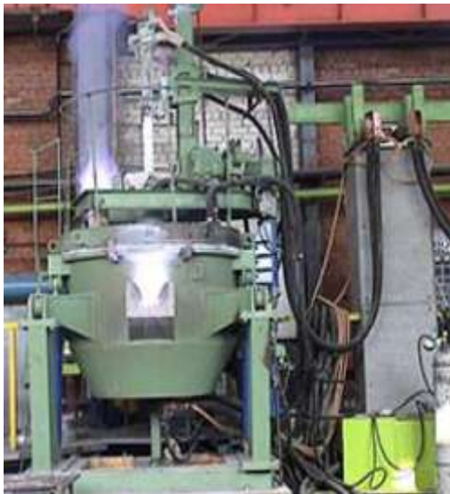
Figure 7. DPPTU-0.5AG direct-current electric arc furnace manufactured by "Ekta" research and production company
