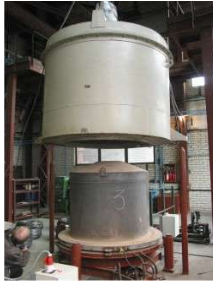
Figure 8. A bell-type furnace manufactured by “Thermoengineering” LLC
