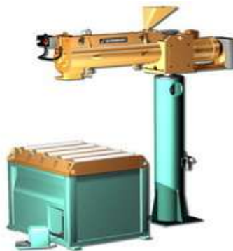
Figure 4. S1Sh3 High-speed single-screw mixer manufactured by "BELNIIIT" OJSC.
