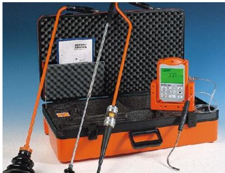
Figure 4. Gas analyzer set used to determine the methane concentration in the tank.
