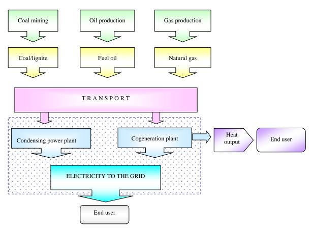
As for the baseline scenarios it was assumed that the Portile de Fier I project output would replace the electricity produced by fuel fired plants, for these plants only direct on site emissions will be taken into account. The GHG emissions resulted from fossil fuels production, transport, etc. as well as downstream emissions are not taken into account.
