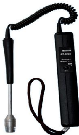
Figure 2. A photo of FT-02V1 leak detector.
