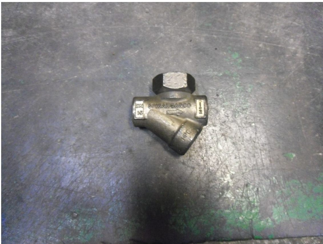
Figure 9 – Condensate drain produced by Spirax Sarco company
