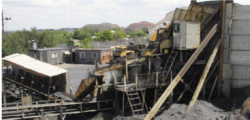
Figure 4 - Location of sifter GIL-52 on industrial site, scraper conveyor SP-202, belt conveyor KLS.
