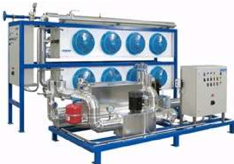
Fig. 3. The system of waste heat recuperators.
