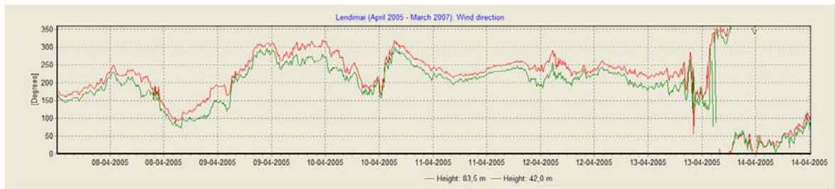
Figure 10. Wind directions on the 83,5 m and 42,0 m wind vane. A difference of around 20 degrees is seen. The 83,5 m wind vane is assumed to be the most correct because the best correlation with long-term reference data is seen for this specific wind vane.
