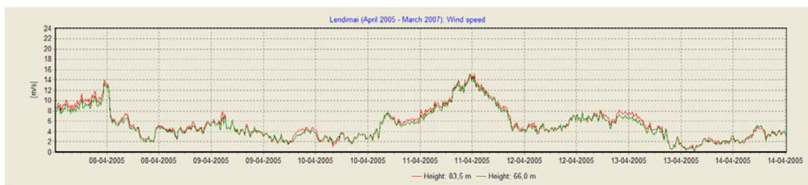
Figure 9. Wind speed measurements at 83,5m and 66,0 m are correlating perfectly
