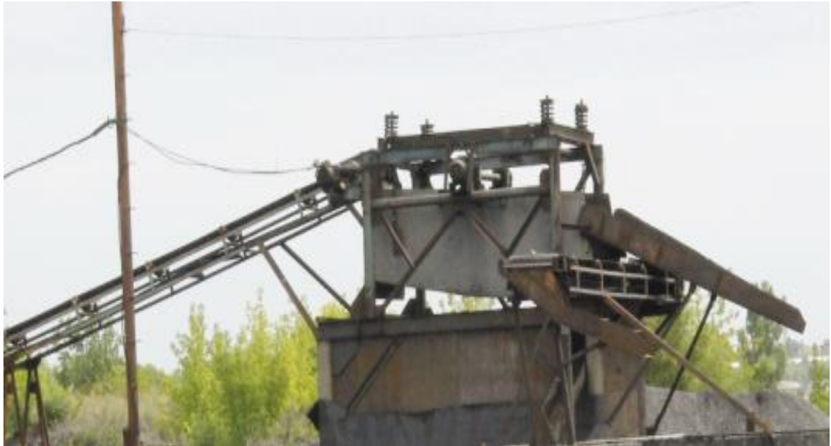
Figure 4 - Machinery for sorting the rock mass
