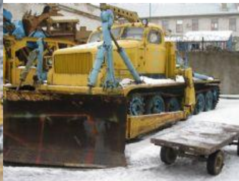
Bulldozer universal BAT-M
