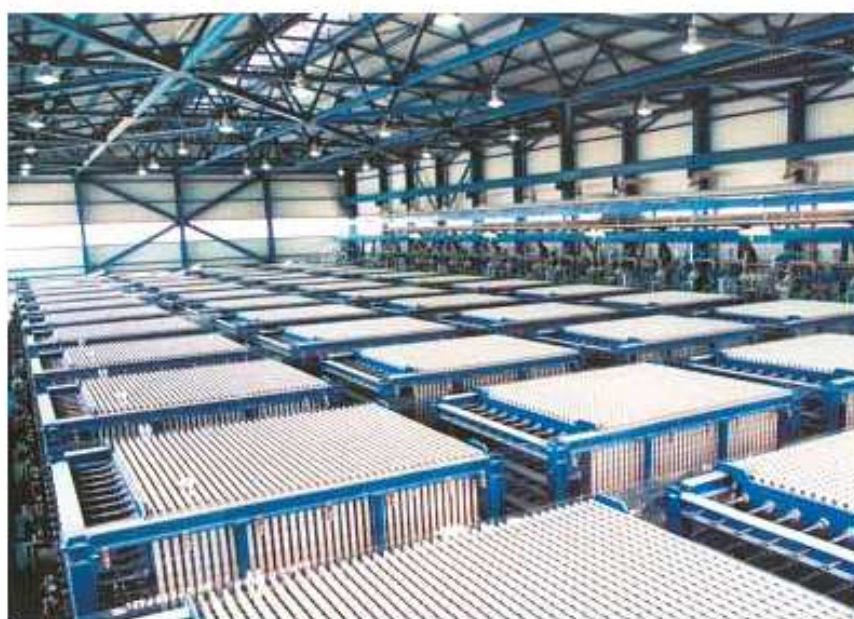
Pic. 4. Caustic soda production unit based on membrane technology.
