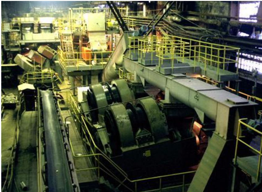
Fig. A.4-3. Modern bark processing line at WPS-3 with Saalasti equipment, 2000
