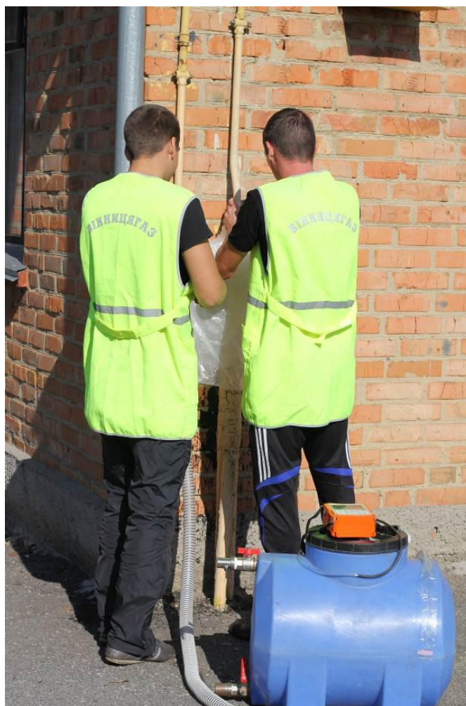
Fig 2. Photo of quantitative measuring of methane emissions device
