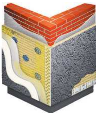
Fig.15. Scheme of thermal insulation of external walls
