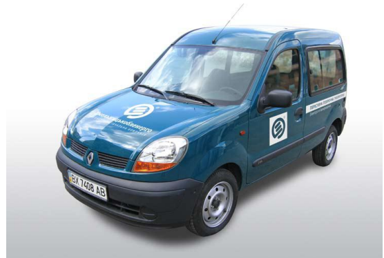
Transportable control laboratory Khmelnytskoblenergo on the basis of the Reno vehicle.
