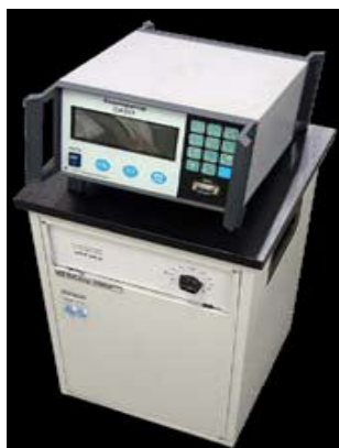
Stationary current transformers control device.
