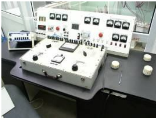
Relay protection service. Stationary control laboratory SCL-10 for the current and voltage transformers control. Post.
