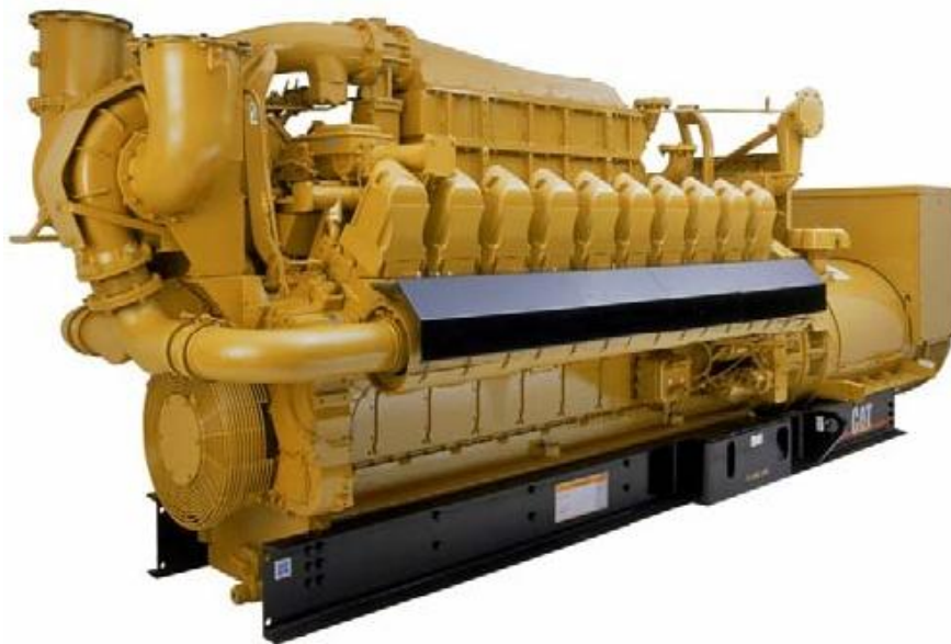
Fig.6. Cogeneration unit produced by "Caterpillar" (USA) G3520B with capacity 1460 kW.
