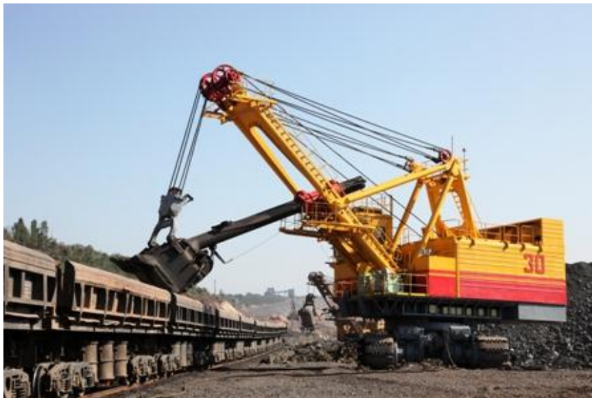
Figure. 7 Excavating machine EGK.
