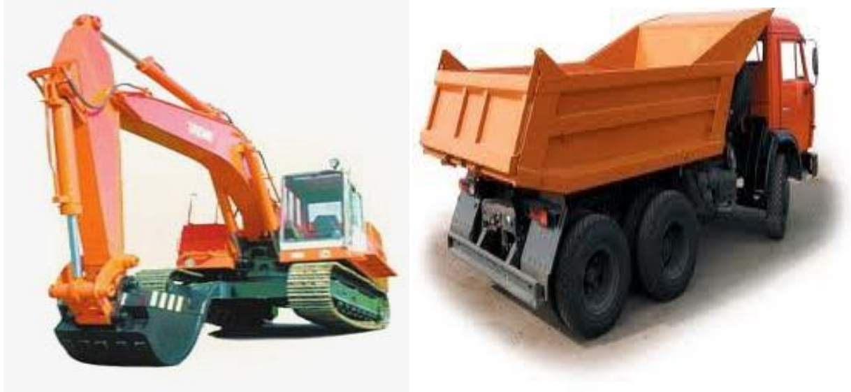
Figure 5 - Special Machinery. Excavator EO-5126, truck Kamaz 55111
