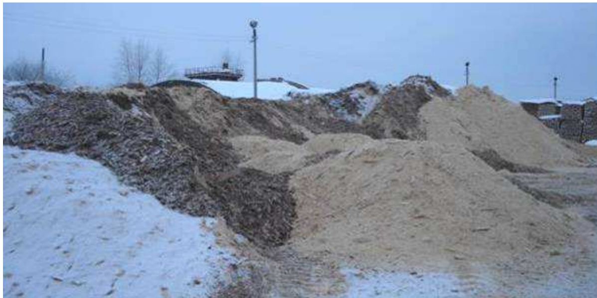
Fig. A.4-8. Bark and wood waste for the new boiler-house in Tsiglomen
