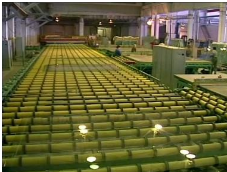
Fig. 8. General view of the cutting machine for float glass.
