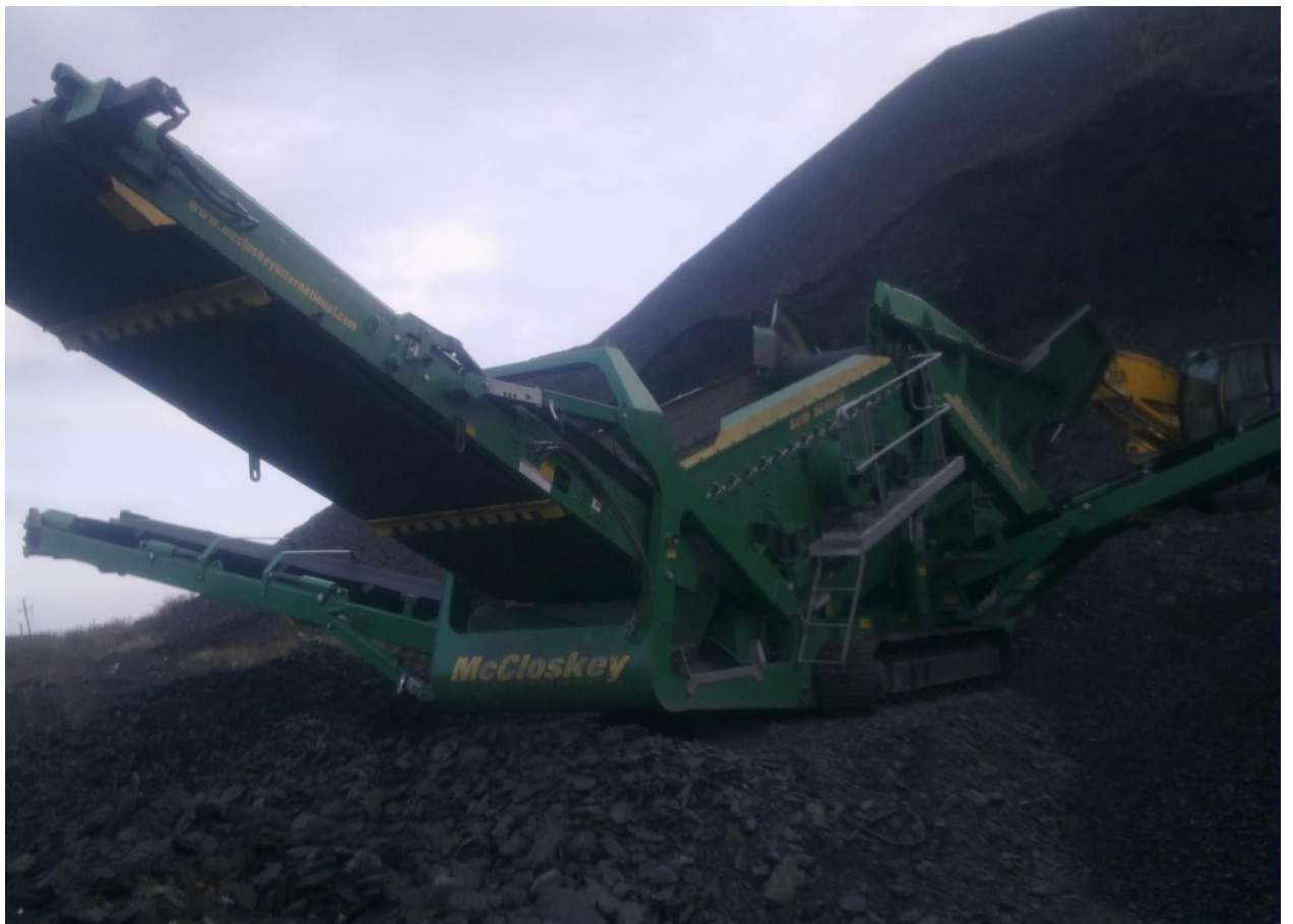
Figure 4 - Machinery for the rock mass sorting
