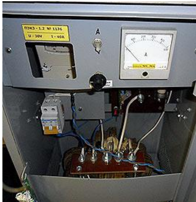
Figure 7. Cathodic protection electric transducer (CPET), produced by "Elkon".
