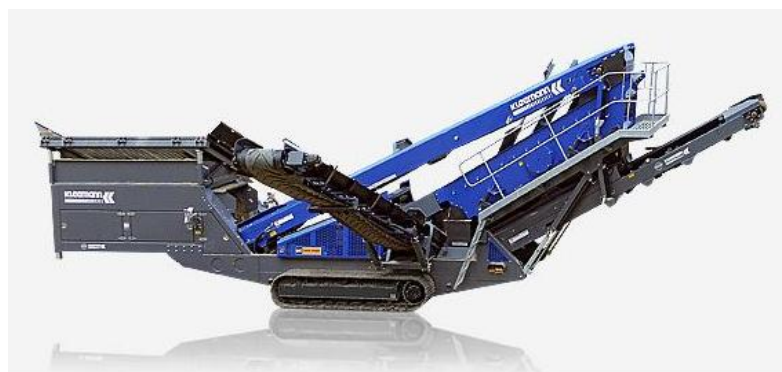
Figure 5 Mobile sorting unit (sieve) Kleemann MS 16Z
