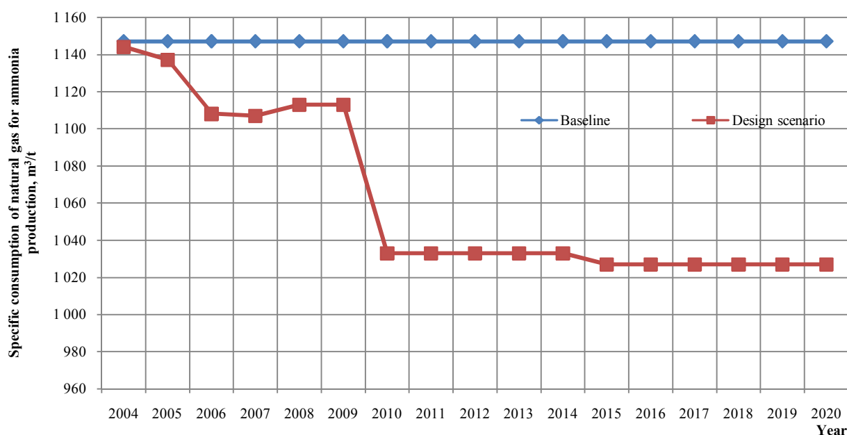
Figure 8 – Expected reduction diagram of natural gas specific consumption for ammonia production unit #2
