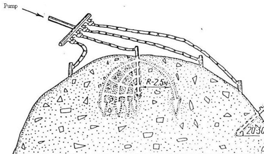
Figure 3 Scheme of antipyrogen pumping with use of several perforated pipes.
