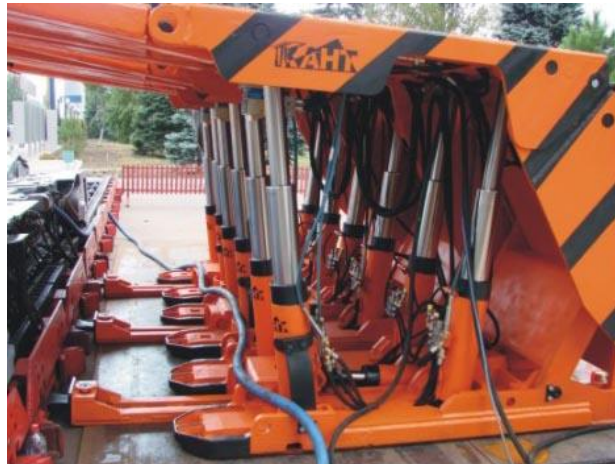
Figure 9. 3KD-90 power roof support Table 5. Specifications of 3KD-90
