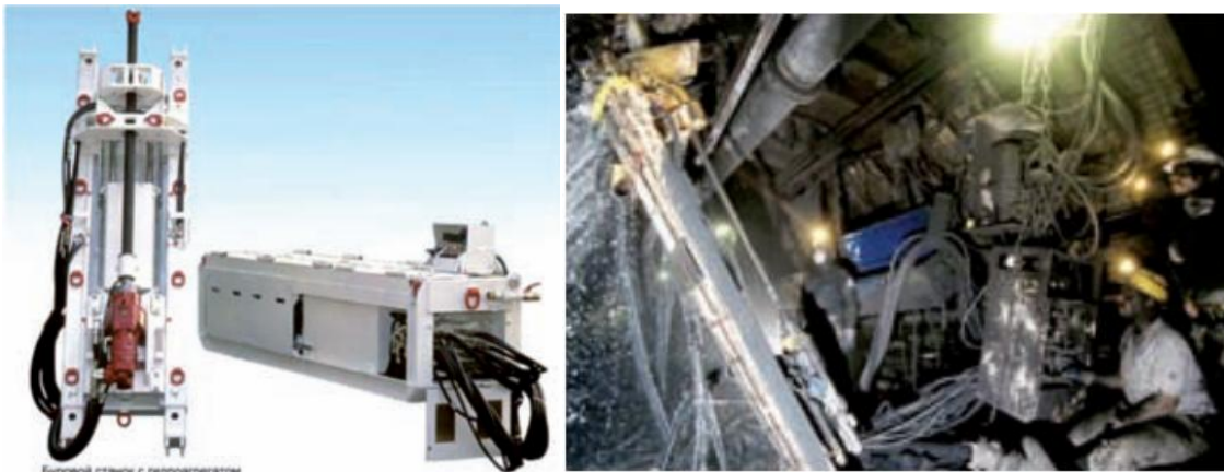
Figure 3. GBH-1/89/12 drilling rig with seam gas drainage manufactured by Deilmann-Haniel mining systems GmbH
