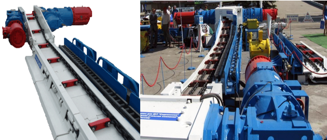
Figure 8. SP 326 mining drag conveyor.
