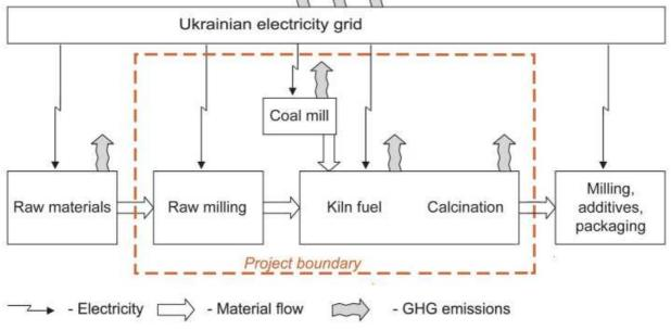
Figure 4: Sources of emissions and project boundary
