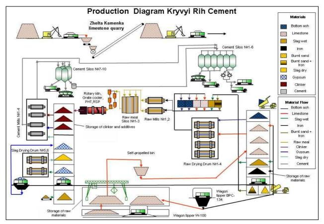
Figure 3: Existing dry process at Kryvyi Rih Cement.
