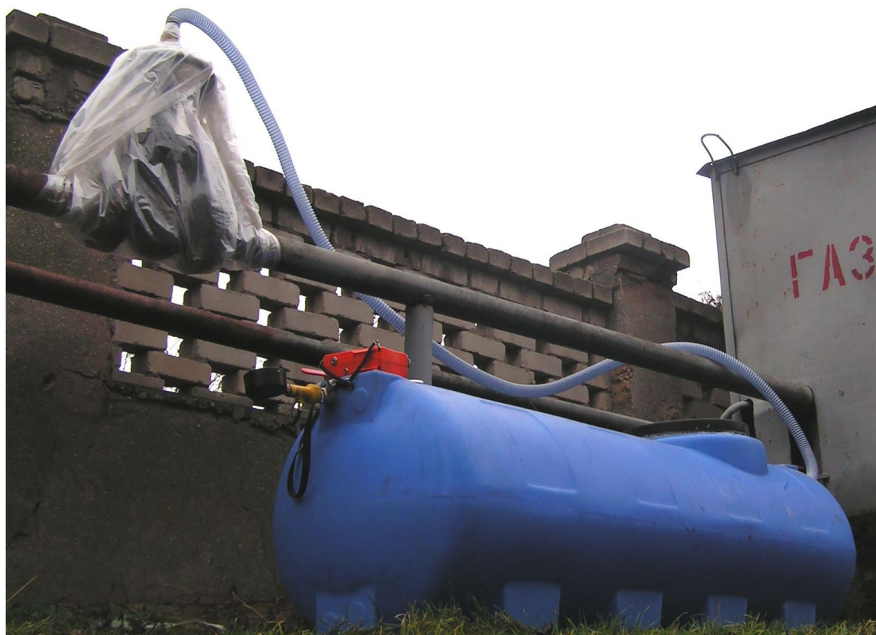
Pic. 3. Photo of a plant for quantitative measurement of methane leakage.
