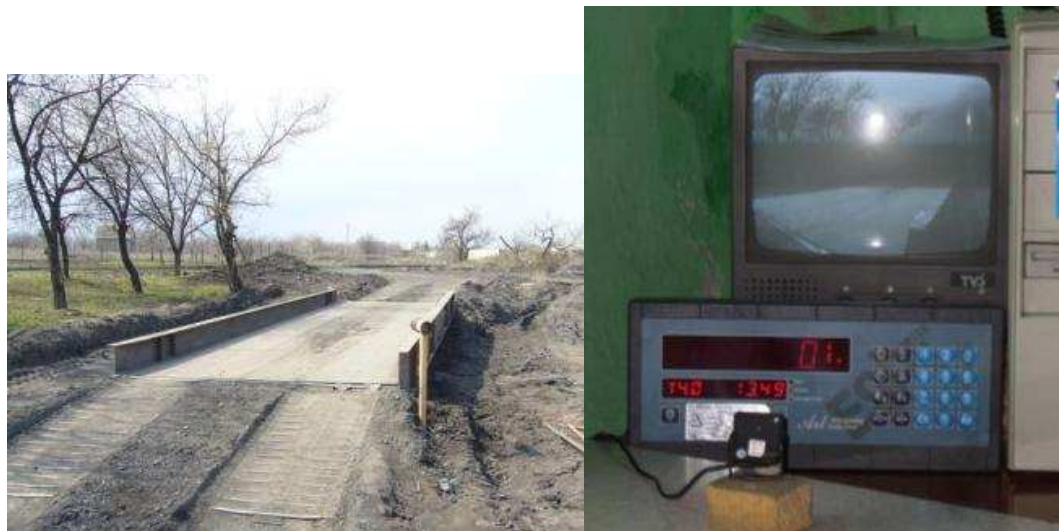
Figure 1 Automobile scales “ББА-40-12”
