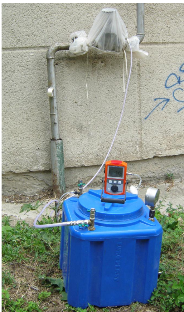
Fig 2. Photo device for quantitative measuring of methane emissions
